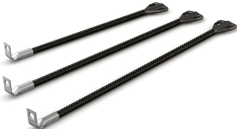
Teplo BF Channel Ties are a range of composite wall ties comprising pultruded basalt fibers set into a resin matrix, with a helical ridge on the bar surface which acts as a drip feature. Each tie has a moulded polymer piece at one end and a crimped stainless-steel piece at the other end. The ties are for use in tying masonry to steel anchor channels which can be face fixed to steel, masonry and timber or embedded in concrete. The ties remove the thermal bridging created by steel ties.
